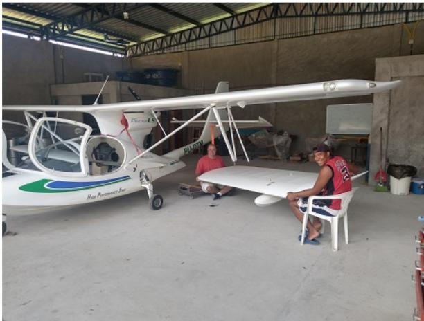
Jimby helps Lloyd and I remove the lower wings to replace the main fuel lines. In May 2018, we replaced all the other rubber parts, but postponed these lines as they are more labor intensive.
